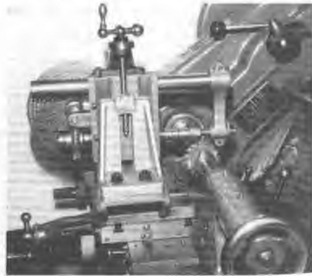
Fig. 57 Another view of the arrangement shown opposite. Even by using a raising block height limitations restrict the size of gear that can be cut.
